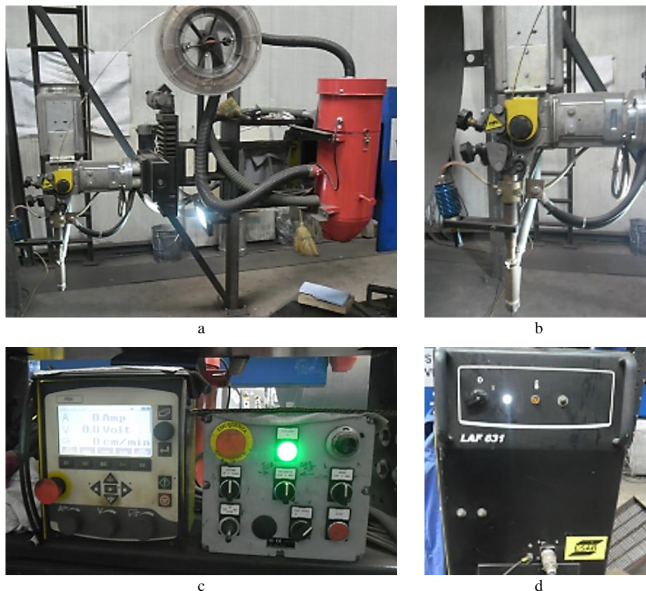
Figure 1 – SAW equipment used for the preparation of welded samples: a – end beam; b – mobile beam; c – control unit PEK-ESAB; d – power source LAF 613-ESAB
