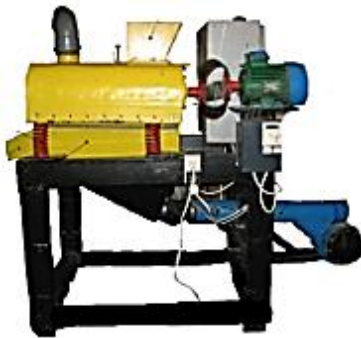
Figure 1 – Laboratory installation and devices for determining the parameters of the walnut drying process: a – laboratory installation for drying walnuts
