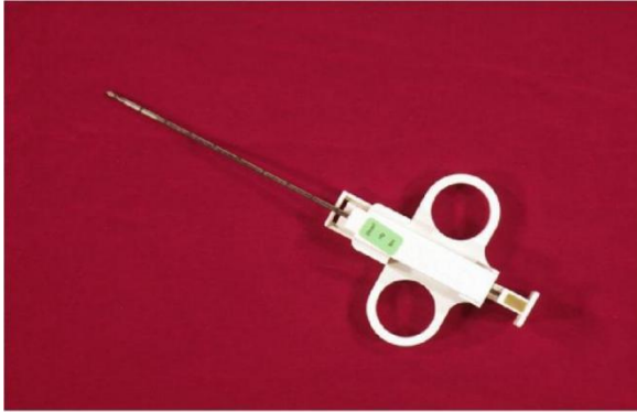
Figure 6 – Biopsy needle for sampling sectional materials
