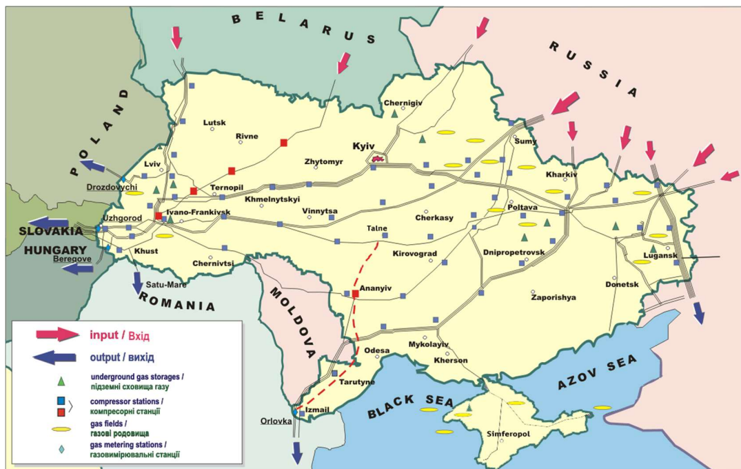
Figure 1.5 – Gas transit pipelines in Ukraine [33]
