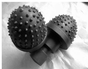
Fig. 7 – The tools for coal cracking strengthened by SDP method
