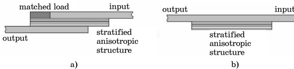
*Fig. 7 – Principle of the construction of optical devices: with transmission (a); with reflection (b)*
