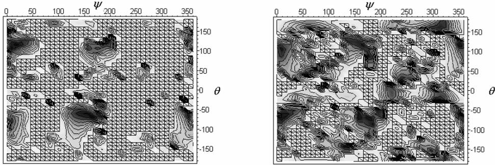
**Fig. 5** – Dependence of the reflection coefficients on the inclination angle of the anisotropy axis and the angle between the incidence plane and the plain containing anisotropy axis for twelve two-layer periods,  $d_2 = 100$  nm,  $d_1 = 40$  nm,  $f = 850$  THz: direct transmission (a); backward transmission (b)
