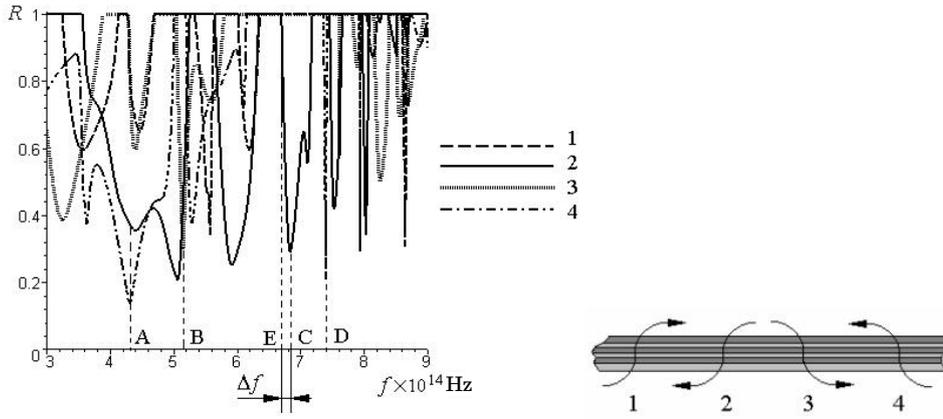
**Fig. 6** – Frequency dependence of the reflection coefficient at  $\theta = 21^\circ$ ,  $\psi = 169^\circ$
