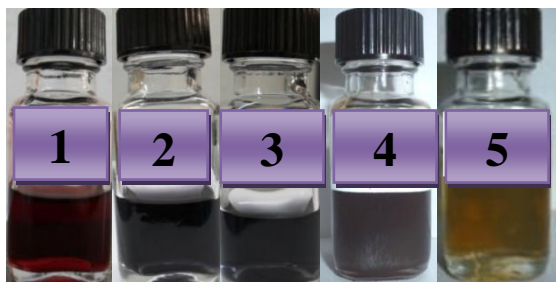
Fig. 1 – Samples of AuNPs stabilized by PVP with M_n = 10 \cdot 10^3 (1), 40 \cdot 10^3 (2) and 350 \cdot 10^3 (3) and AgNPs protected by PVP in DMF (4) and DMSO (5)
