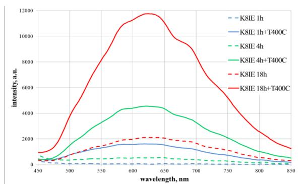
**Fig. 3** – Luminescence spectra K8 samples depending on the time of ion exchange and subsequent heat treatment at temperature  $T = 400\text{ }^{\circ}\text{C}$ . Excitation wavelength  $\lambda = 405\text{ nm}$ .
