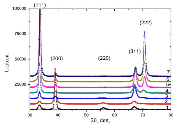
**Fig. 2** – Plots X-ray diffraction spectra of coatings ZrN, obtained by  $P_N = 0,65$  Pa,  $U_{ip} = 0$  V,  $U_b$ : 1 –  $-27$  V; 2 –  $-40$  V; 3 –  $-70$  V; 4 –  $-100$  V; 5 –  $-150$  V; 6 –  $-220$  V; 7 –  $-300$  V
