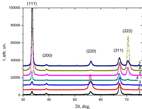
**Fig. 3** – Plots X-ray diffraction spectra of coatings ZrN, obtained by  $P_N = 0,65$  Pa,  $U_{ip} = -1200$  V and  $U_b$ : 1 – – 27 V; 2 – – 40 V; 3 – – 70 V; 4 – – 100 V; 5 – – 150 V; 6 – – 220 V; 7 – – 300 V
