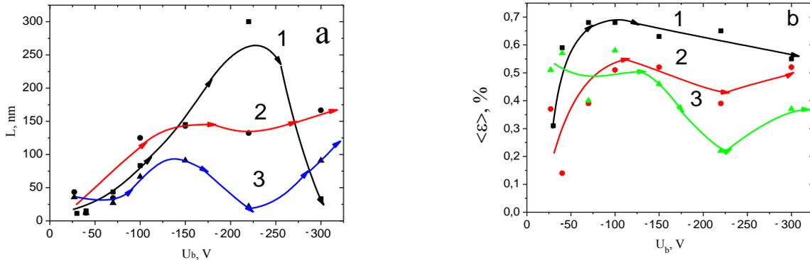
**Fig. 6** – The dependence of the crystallite size (a) and microstrain (b) from the constant potential at  $P_N = 0,65$  Pa: 1 –  $U_{ip} = 0$  V; 2 –  $U_{ip} = -1200$  V; 3 –  $U_{ip} = -2000$  V
