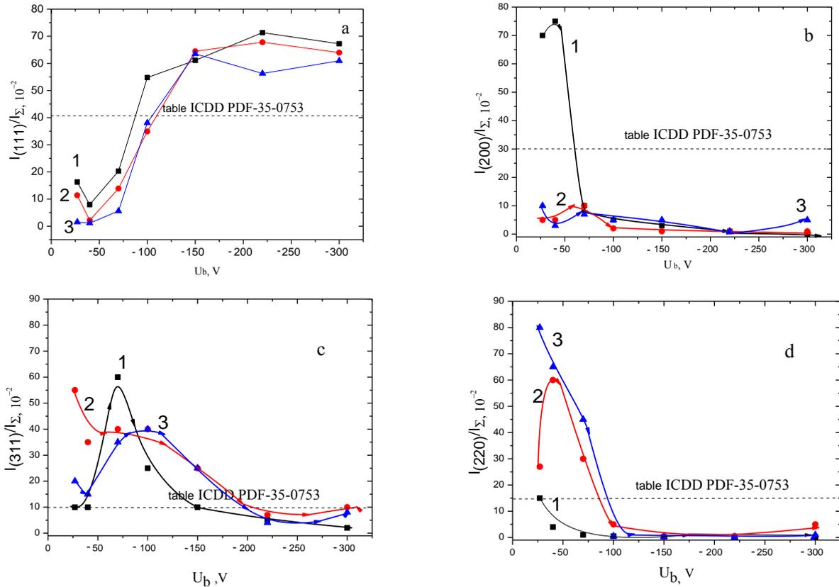
**Fig. 5** – Depending on the parameter of texture  $P_{hkl}$  from values  $U_b$  for different planes: a – (111), b – (200), c – (311), d – (220); 1 –  $U_{ip} = 0$  V, 2 –  $U_{ip} = -1200$  V, 3 –  $U_{ip} = -2000$  V
