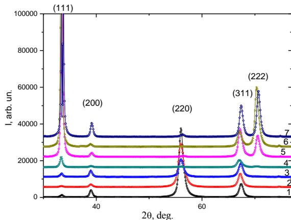
**Fig. 4** – Plots X-ray diffraction spectra of coatings ZrN, obtained by  $P_N = 0,65$  Pa,  $U_{ip} = -2000$  V and  $U_b$ : 1 – – 27 V; 2 – – 40 V; 3 – – 70 V; 4 – – 100 V; 5 – – 150 V; 6 – – 220 V; 7 – – 300 V
