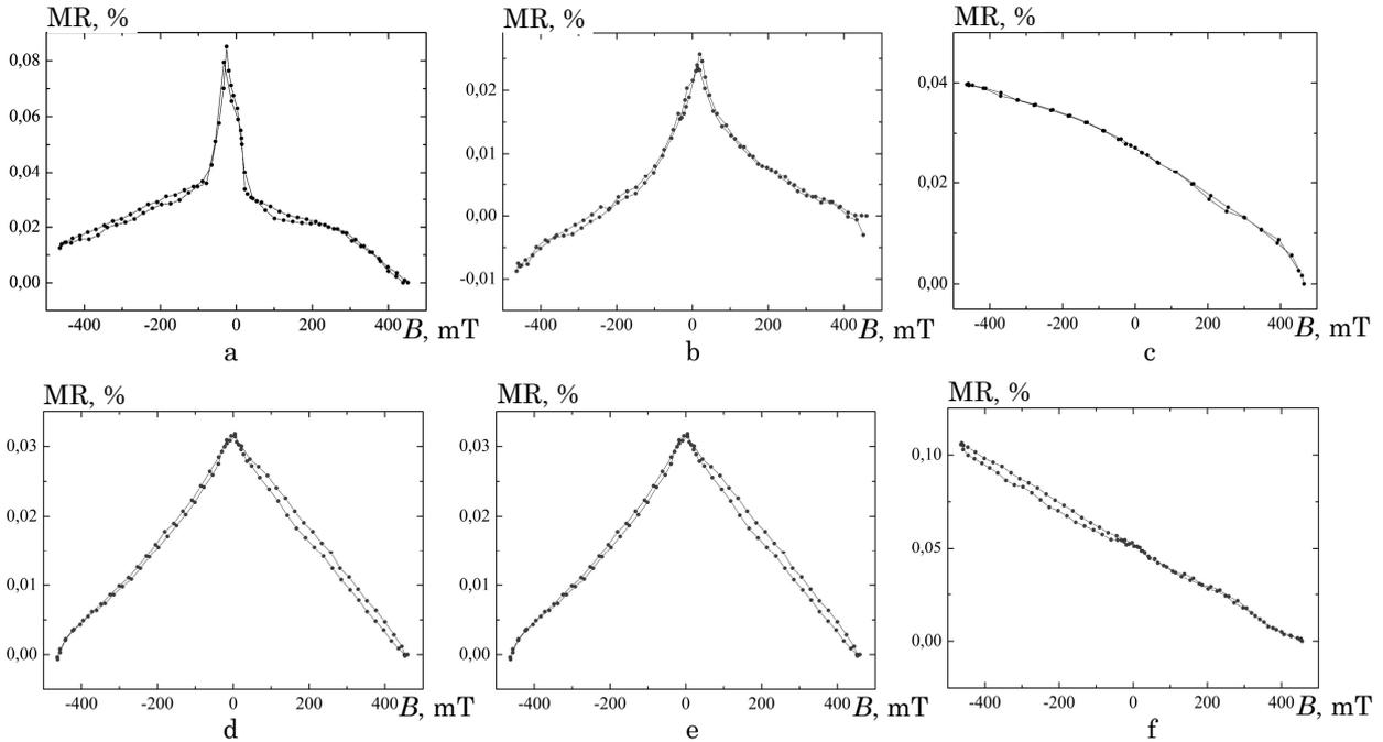
**Fig. 3** – Dependence of the MR value on the magnetic induction for the unannealed (a-c) and annealed to 870 K (d-f) system Fe(10)/Ge(8)/Fe(20)/S for the longitudinal (a, d), transverse (b, e) and perpendicular (c, f) measurement geometries
