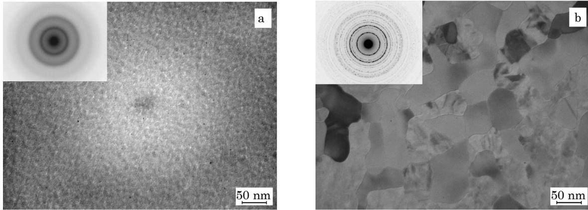
**Fig. 2** – Microstructure and the corresponding electron diffraction patterns from single-layer Ge(20) films obtained at  $T_s = 420$  K (a) and  $T_s = 800$  K (b). Film thickness in nm is given in the brackets
