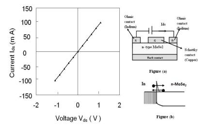
**Fig.** 2 – Drain –Source I-V characteristics of n-type  $MoSe_2$  MESFET. Inset figures (a) show the contacts to the n-type MoSe2 channel and (b) tunnelling of electrons across the In-nMoSe<sub>2</sub> Ohmic interface
