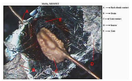
Fig. 1 – A typical optical micrograph (20X) of MoSe<sub>2</sub> MESFET
