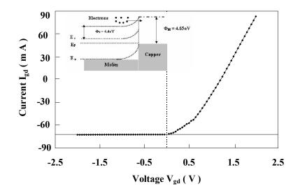
**Fig. 3** – I-V characteristics of the metal semiconductor Schottky junction formed by the copper gate on the n-type  $MoSe_2$  channel. The inset figure is energy band diagram of n-type  $MoSe_2$  and Cu
