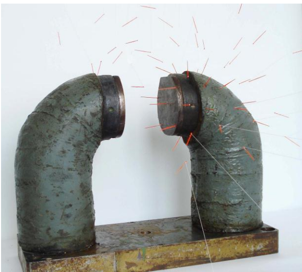
Fig. 1 – The magnet system: radius of cylindrical magnets 55 mm, height of cylinder 40 mm, where length of visible magnetic part 9 mm. The width of gap: 91 mm. Light steel needles free hanged by length fibers are arranged along magnetic induction lines visualizing them
