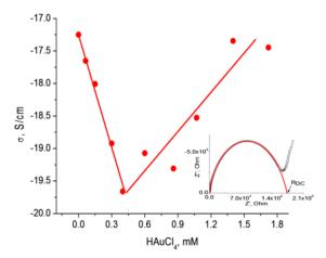
Fig. 3-DC conductivity of CS / AuNP's films as a function of the of the HAuCl<sub>4</sub> concentration obtained from impedance measurements at room temperature. Insert shows complex impedance spectra
