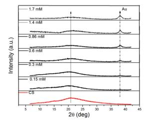
Fig.  $1-\mbox{XRD}$  pattern of films obtained from solution with different  $HAuCl_4$  concentration
