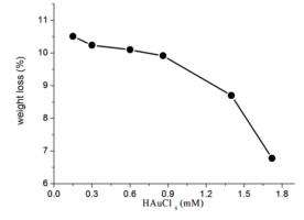
Fig. 2 - Dependence of water content on HAuCl<sub>4</sub> concentration
