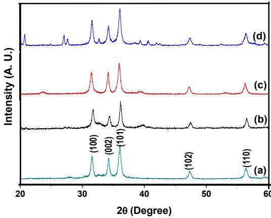
**Fig. 1** – XRD pattern of undoped and Cu doped ZnO [(a) undoped ZnO, (b) 2 %, (c) 4 % and (d) 6 % Cu doped ZnO]
