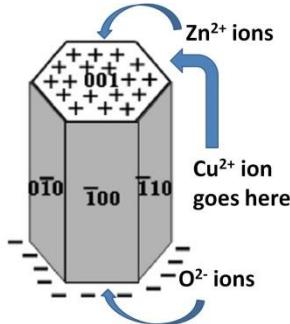
**Fig. 2** – Schematic of the Cu doping in ZnO crystal
