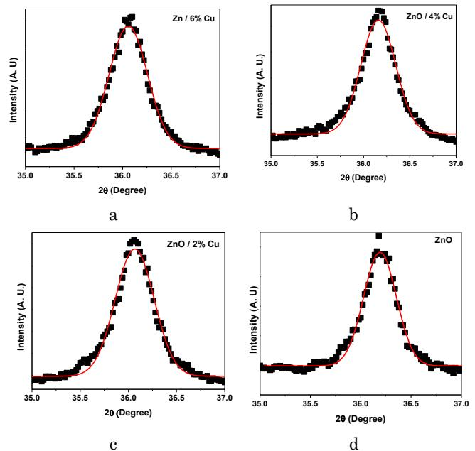
**Fig. 3** – Gaussian fitting of (101) peak of undoped and Cu doped ZnO
