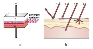
**Fig.** 1 – Structure of a diode laser (a); processes in biological tissue under the influence of laser radiation (b): 1 - reflection; 2 - absorbtion; 3 - transmission, 4 - scatter
