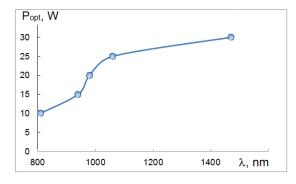
Fig. 2 – Experimental dependences of the output optical power of a diode laser versus the working wavelength of laser radiation with stepwise adjustment of power
