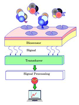
Fig.  $1-{\rm Diagram}$  of the structure and operating principle of biosensors
