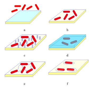
Fig. 3 – Methods used for bioreceptor immobilization in biosensors: before immobilization (a), adsorption (b), covalent binding (c), matrix entrapment (d), cross-linking (e), encapsulation (f)
