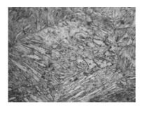
Figure 6 – Microstructure of steel X40CrMoV5-1-1 after hardening from 1070 °C (needle martensite, austenite residual and carbides), x500
