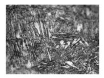
Figure 7– Microstructure of steel 30WCrV17-2 after hardening from 1080 °C (needle martensite, austenite residual carbides), x500
