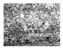
Figure 8 – Microstructure of steel X40CrMoV5-1-1 after hardening and double tempering (tempering troostite), x500
