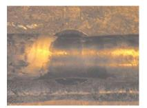
Figure 3 – The wear of the needle-mandrel pipe press [3]
