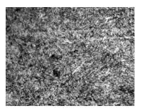
Figure 9 – Microstructure of steel 30WCrV17-2 after hardening and double tempering (tempering troostite), x500
