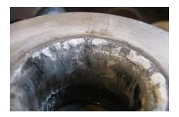
Figure 1 – The wear of the matrix for the pipe press [5]
