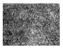
Figure 4 – Microstructure of steel X40CrMoV5-1-1 after hardening from 1070 °C and tempered at 550–570 °C (1st temper), 530–550 °C (2nd troostit temper), x500 [8]
