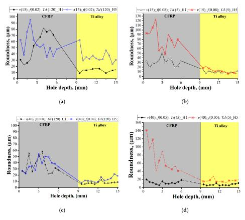
**Figure 8.** The effect of the time delay factor on hole roundness. (**a**,**c**) Comparison of hole roundness for holes No. 1 and No. 5 drilled under CDM conditions; (**b**,**d**) comparison of hole roundness for holes No. 1 and No. 5 drilled under HDM conditions.
