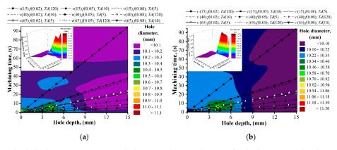
**Figure 6.** The hole diameter measures in hole No. 1. (**a**) Distribution of hole diameter under the conditions of the machining time and hole depth for hole No. 1; (**b**) distribution of the hole diameter in terms of machining time and hole depth for hole No. 5.
