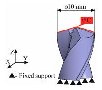
Figure 1. Schematic illustration of the FE model of a drill.
