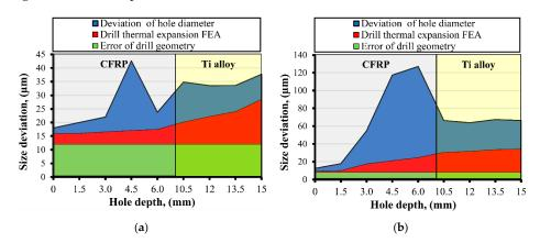
**Figure 7.** Hole diameter measured in hole No. 1. (a) Components of hole diameter deviation for hole No. 1 trail No. 2 (v (15); f (0.05);  $T_d$  (120)); (b) components of hole diameter deviation for hole No. 1 trail No. 7 (v (65); f (0.02);  $T_d$  (5)).
