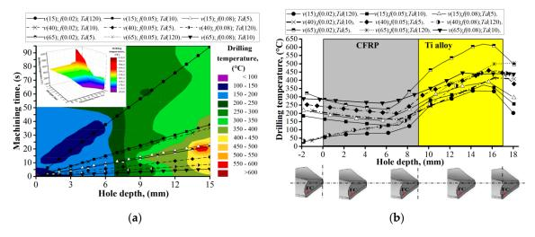
**Figure 5.** Drilling temperature when machining hole No. 5 in the CFRP/Ti alloy stack. (**a**) Distribution of the drilling temperature with respect to machining time and hole depth; (**b**) drilling temperature evaluation of the hole depth.
