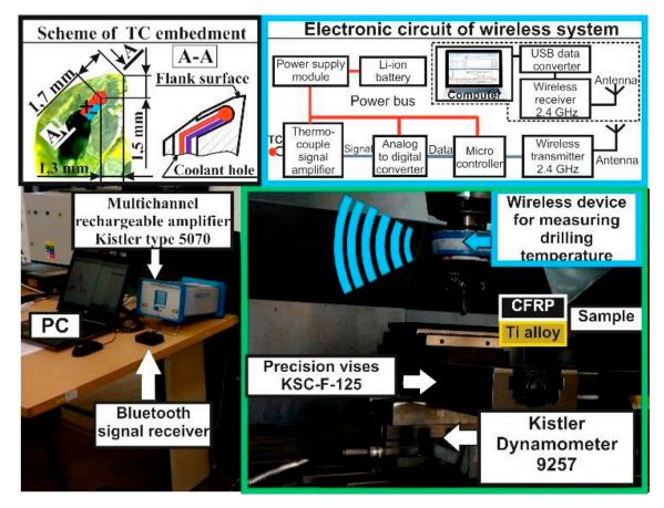
Figure 3. Experimental setup of the drilling tests.
