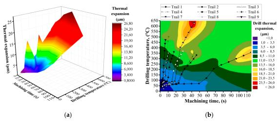
**Figure 2.** Results of finite element modeling of drill thermal expansion. (a) evaluation of drilling thermal expansion depending on machining time and drilling temperature; (b) Drill thermal expansion Plane Projection.
