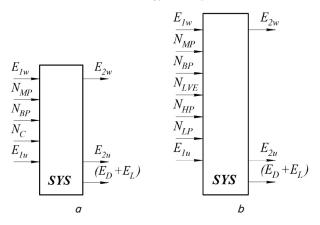
Fig. 4. The scheme of the exergetic transformations: *a* is the traditional heat pump installation; *b* is the LVE-based installation
