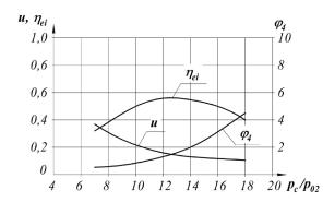
Fig. 1. The graph of the dependence of the degree of overproduction of steam  $\psi_4$ , the injection coefficient and the effective efficiency  $\eta_{ei}$  on the magnitude of the increase in the pressure of the passive flow  $\rho_c/\rho_{02}$  at  $t_{01}$ =121-149 °C,  $\rho_{01}$ =300-500 kPa, and  $\rho_{02}$ =5 kPa
