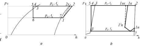
Fig. 3. A comparison of the cycles: *a* is the traditional VCHP with a scroll compressor; *b* is based on the LVE
