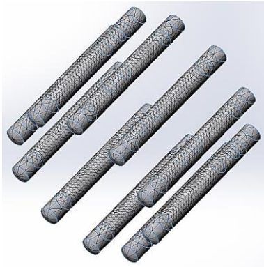
Figure 11 – Slow speed shaft rollers with FEM grid control applied
