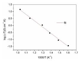
Fig. 6 – Electrical conductivity versus 1000/T of the PGDC sample
