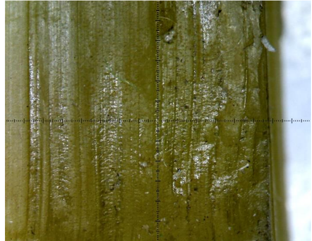
Fig. 7 The friction surface of the BPU based on OEBGA 2000 in water at P_c = 11-24\%
