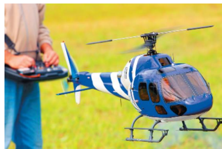
Figure 7.9 - The battery pack in this radiocontrolled helicopter contains 2.4 \times 10^4 J of electric energy. When this energy is used up, the internal energy of the battery pack decreases by this amount, so \Delta U_{\text{int}} = -2.4 \times 10^4 J. This energy can be converted to kinetic energy to make the rotor blades and helicopter go faster, or to gravitational potential energy to make the helicopter climb
