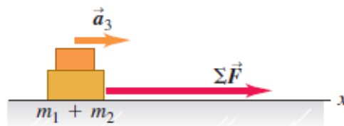
Figure 4.10 - For a given net external force \Sigma \vec{F} acting on an object, the acceleration is inversely proportional to the mass of the object. Masses add like ordinary scalars
