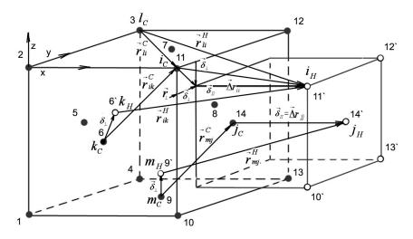
Fig. 1 - Diagram of the forces, acting in the sections of deformed cell
