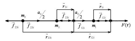
**Fig. 3** – Forces action on the reduced masses in an arbitrary time moment under the external force  $\vec{F}(\tau)$  influence. Dots denote the initial positions of reduced masses in a cell; asterisks present the positions of reduced masses in a cell in an arbitrary time moment
