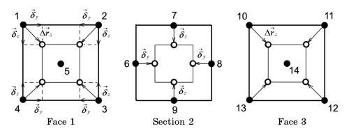
Fig. 2 – Schematic representation of the deformation vectors directions
