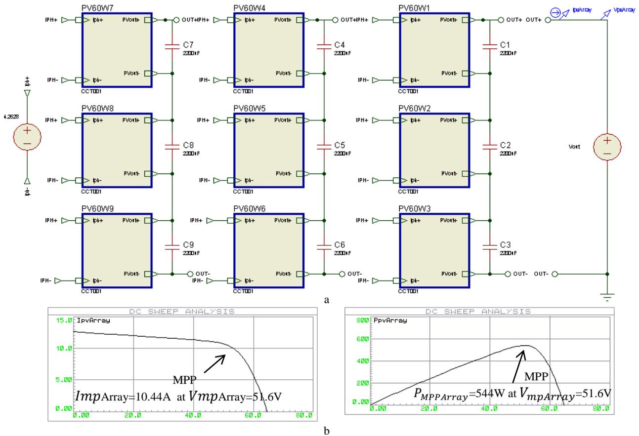
Fig. 13 – PV Array Model a, Current  $I_{pV}$  and Power  $P_{pV}$  Curves b.
