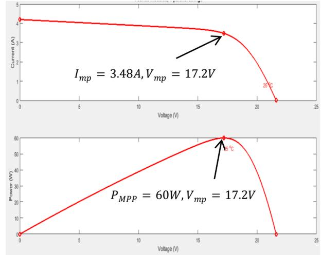
Fig. 5 – I-V and P-V curves of a 60 W – 17.2 V PV at STC
