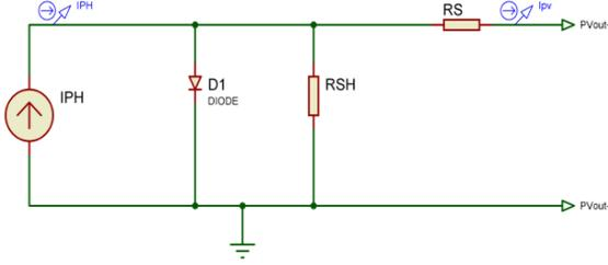
Fig. 2 – illustrates circuit of PV solar cell.
