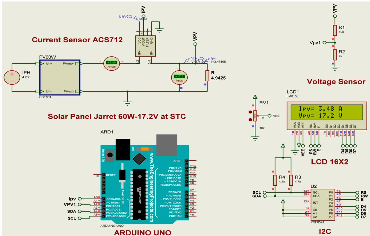
Fig. 14 – Shows the simulation PV model using Proteus and Arduino.
