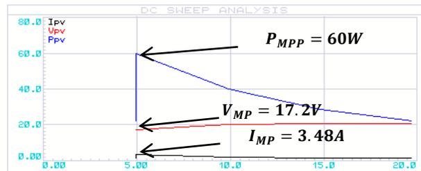
Fig. 16 – Shows current, voltage, and power curves according to resistance  $R_{load}$ .
