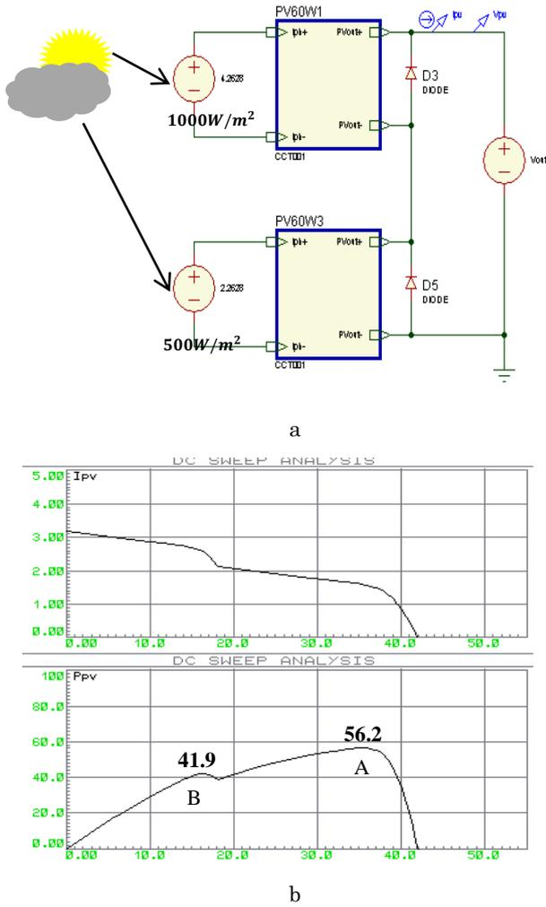
Fig. 12 – shows sub-circuit *a*, characteristics of the PV panel under irregular irradiation *b*.
