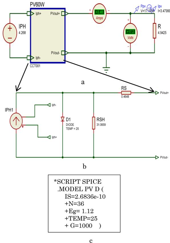
Fig. 6 – Present sub-circuit model under Proteus (a), corresponding circuit based on a single-diode model (b), SPICE code (c)
