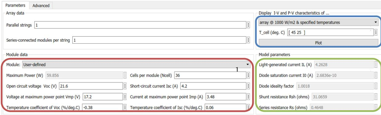
Fig. 4 – Block Parameters PV module of Jarett 60 W – 17.2 V under Matlab/Simulink tools
