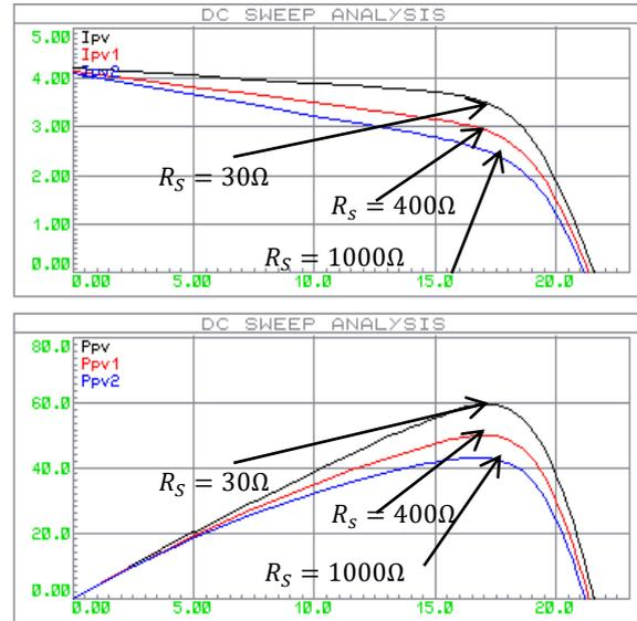
Fig. 11 – Shows  $I_{pV}$  and  $P_{pV}$  curves for different values of  $R_{sh}$ .
