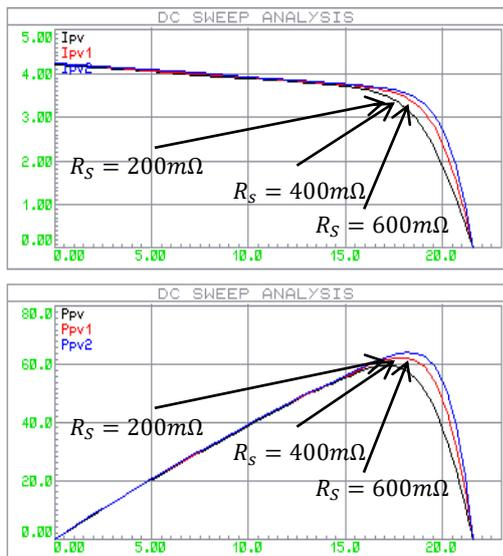
Fig. 10 – Shows  $I_{pV}$  and  $P_{pV}$  curves for different values of  $R_s$
