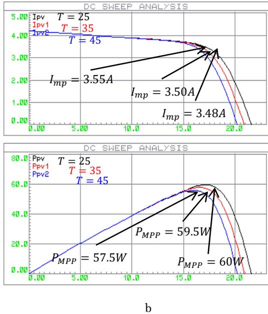
Fig. 9 – shows the sub-circuits (a),  $I_{pV}$  and  $P_{pV}$  curves characteristics at different temperature settings using Proteus software (b)
