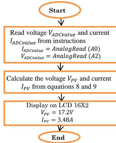
Fig. 15 – Algorithm of the system used to measure the current  $I_{pV}$  and Power  $P_{pV}$ .
