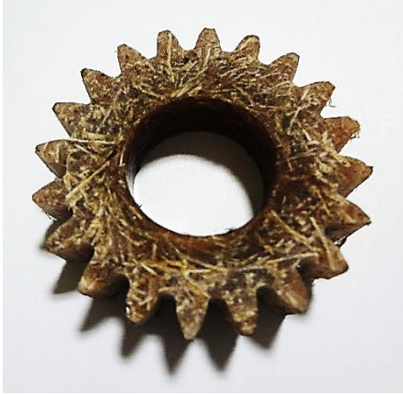
Figure 3 – PPLSF composite gear
