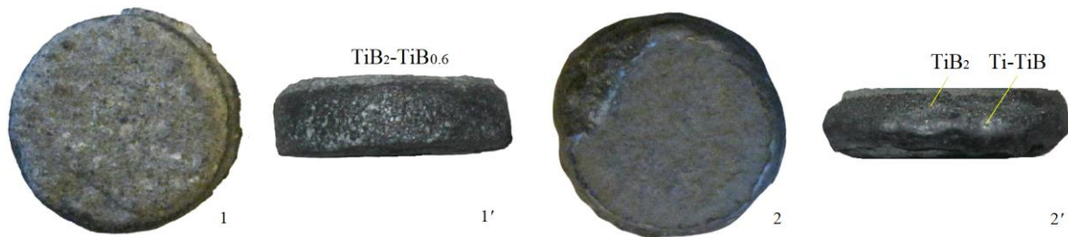
Figure 2 – A round disk-shaped sample obtained by SHS compaction in a vacuum with accompanying Joule heating (top and side views): 1–1' – sample without overheating (duration of Joule thermostating is 1.5 min at a pressing pressure of 150 MPa); 2–2' – the same after overheating up to 1800–2000 °C (duration of thermostating is 3.5 min)
